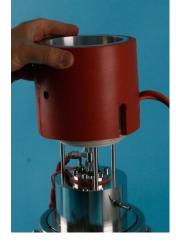
Beaker 3L with jacket for hardening solution
