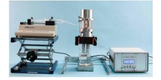
Lord Rayleigh has developed the following theory in the year 1878: A laminar jet of liquids falls apart into drops of equal size, if you superimpose a vibration with a wave length, longer than the girth of the undisturbed jet on the liquid. In order to superimpose the vibration either you can vibrate the nozzle itself or you can superimpose the vibration on the liquid with a suitable device before it passes the nozzle. Our single nozzle units use the first possibility.
