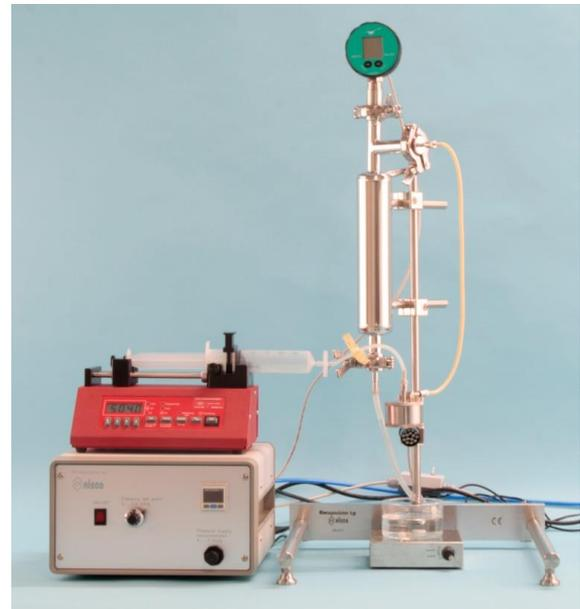
The bead generator with coaxial airflow is basically made of stainless steel 1.4435 (equivalent 316L) and can withstand most chemicals and high temperatures, which make the unit very suitable for any disinfecting/cleaning method including autoclave cleaning. As gaskets O-rings made of EPDM are delivered. For pharmaceutical or medical applications the required material certificates are available.
