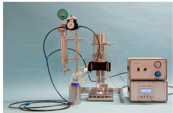
During the work with very low pressure the drops won't be produced, but there will be a laminar jet smaller than the nozzle applied. If the vibration would be superimposed the even sized beads down to half the size of the applied nozzle could be produced.
