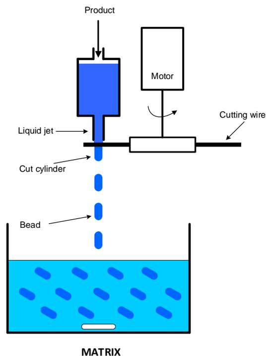
The size of the beads can be adjusted within a range of between approx. 200 µm up to several millimetres.
