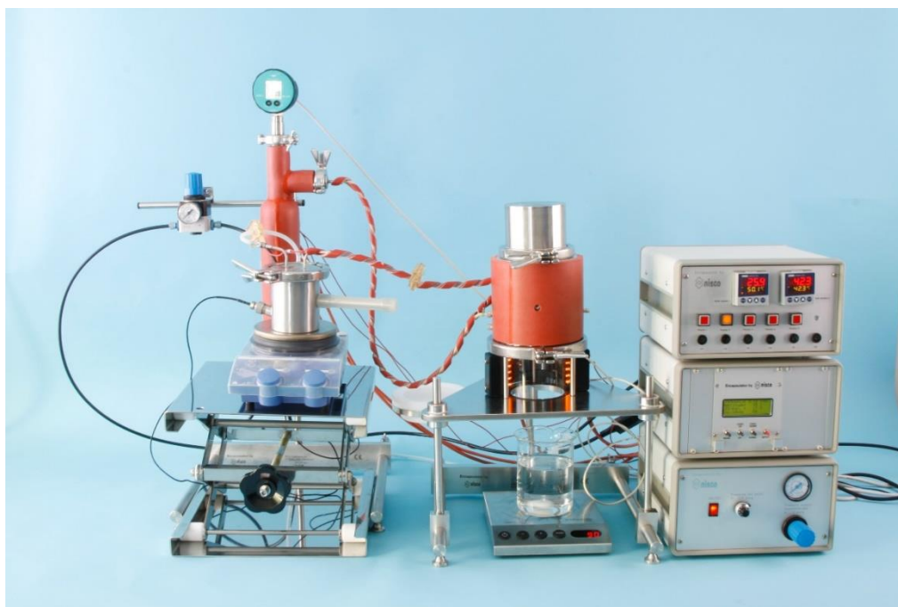
Fig. 16: Typical setup for microencapsulation with gelatin (VARD2Go . Aerodynamic Thermal Option)
