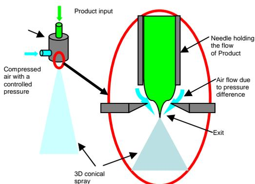
The product enters through a central needle. The exit orifice, which is centrally in line with the axis of the needle, has been counter sunk externally. The counter sunk leads to the aerodynamical effect that the jet has the smaller diameter when it is passing the orifice than the needle. The needle is enclosed in a pressure chamber with an exit through the orifice. The size of the drops is determined by the product flow rate and the pressure inside the chamber.
