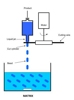
The size of the beads can be adjusted within a range of between approx. 200 m up to several millimetres.
