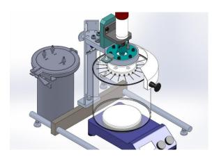
As only a mechanical cut and the subsequent bead shaping driven by the surface tension are responsible for bead generation, the viscosity of the fluid has no direct influence on the bead formation itself. Thus, the jet cutting technology is capable of processing polymers with viscosities up to several thousand mPas (for example: alginate,
