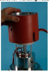
Beaker 3L with jacket for hardening solution
