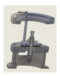
For work with two different liquids **coaxial 6 nozzle head** is available.
