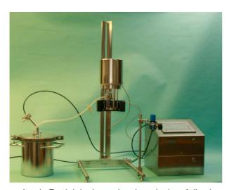
Lord Rayleigh has developed the following theory in the year 1878: A laminar jet of liquids falls apart into drops of equal size, if you superimpose a vibration with a wave length, longer than the girth of the undisturbed jet on the liquid. In order to superimpose the vibration either you can vibrate the nozzle itself or you can superimpose the vibration on the liquid with a suitable device before it passes the nozzle. Our single nozzle units use the first possibility.
